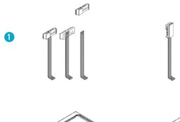
The support bracket clip can be inserted horizontally or upright. This reduces the number of parts to a minimum.
